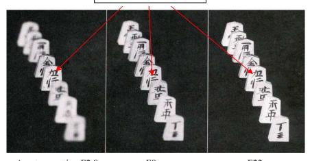
Aperture setting F2.8F8F22The photograph taken with F22 appears in sharp image compared to the one with F2.8.However, too small aperture causes deterioration in resolution.
